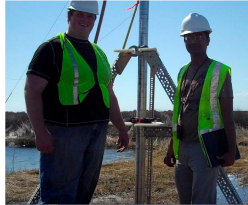
Figure 14. Location of Breach Along NC-12 and Set Up for Testing Using ISEEP
