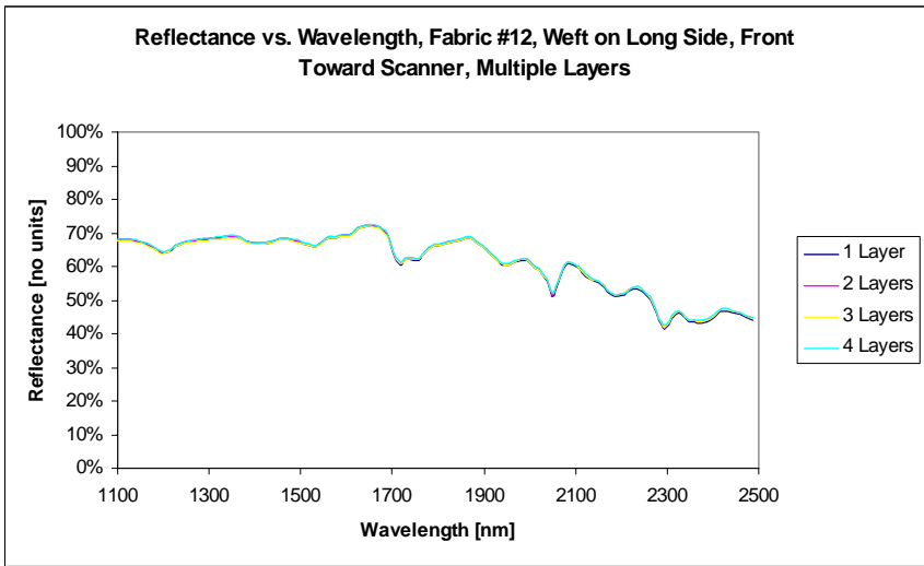
Figure A-12 Multiple Layer And Front vs. Back Comparisons For Fabric #12
