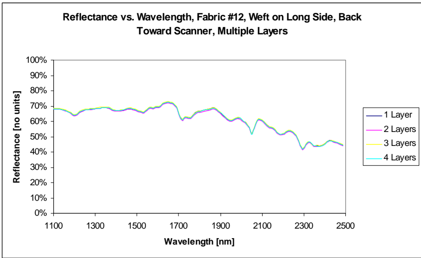
Figure A-12 Multiple Layer And Front vs. Back Comparisons For Fabric #12
