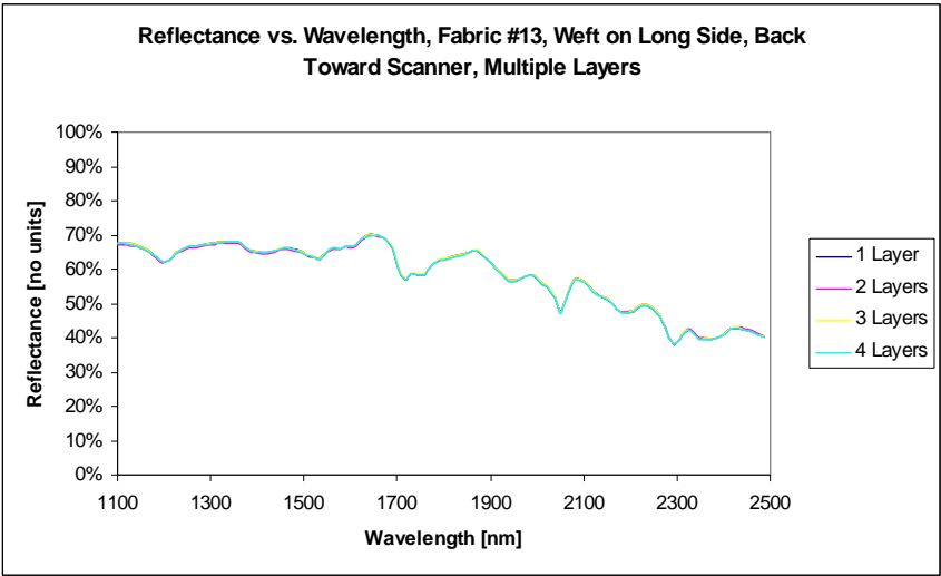
Figure A-13 Multiple Layer And Front vs. Back Comparisons For Fabric #13
