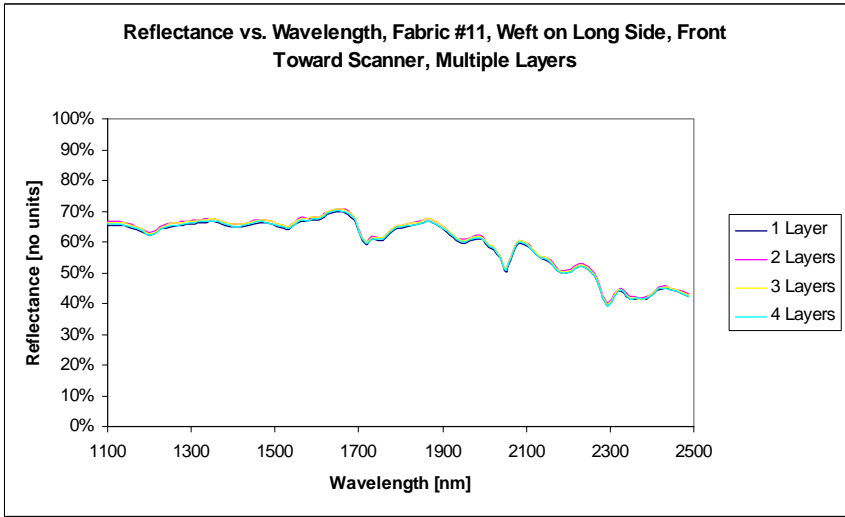
Figure A-11 Multiple Layer And Front vs. Back Comparisons For Fabric #11
