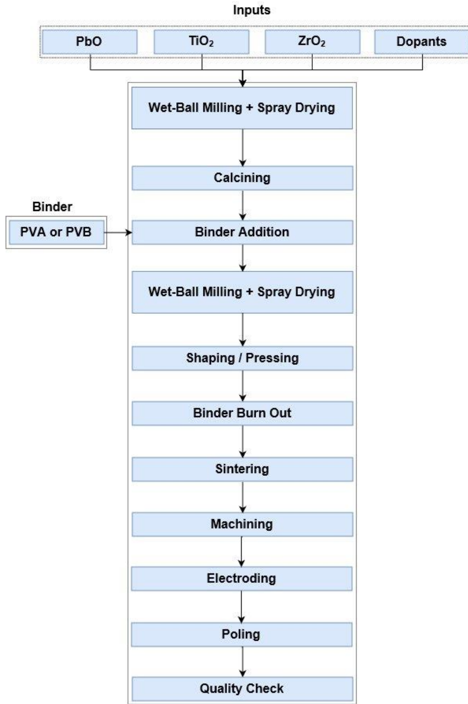
Figure 3.3 Commercial PZT manufacturing process.
