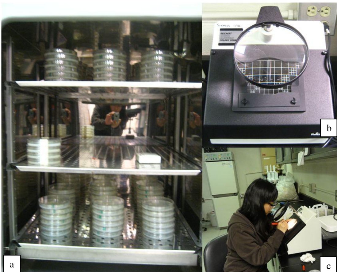
[a] Plates in the incubator; [b] colony counter [c] counting the colony with the counter
