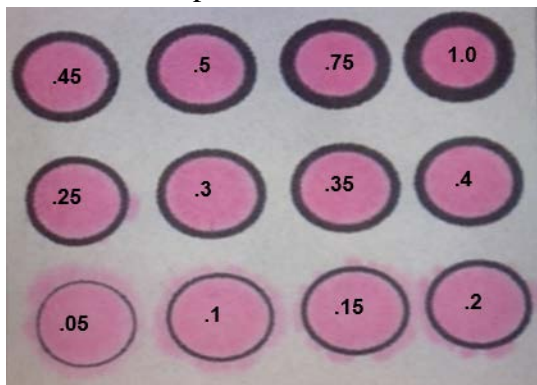
Figure 2.5: Walls of varying thicknesses printed wax thickness from 0.05 mm to 1 mm (0.05 mm increments between .05 mm and .5 mm and .25 mm increments between .5mm and 1 mm) were created and loaded with equal volumes of dilute R6G dye in 50/50 Water/Methanol solution to determine minimal containment thickness.
