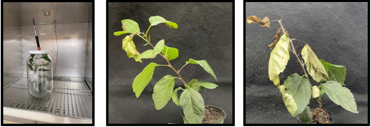
Fig. 4-1: Headspace analysis of ethanol using SPME of apple seedlings inoculated with E. amylovora Ea110. (a) 4 L glass jar with an apple seedling and SPME fiber inserted through rubber septum fitted in lid, (b) apple seedling 7 DAI with wilting and interveinal necrosis, and (c) apple seedling 14 DAI with leaf necrosis and wilting.
