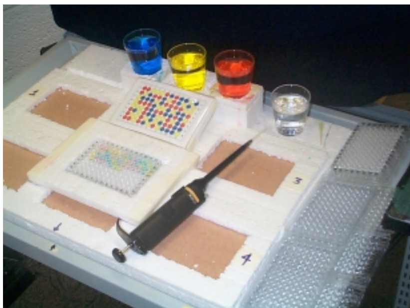
Figure 8-2. Close-up view of pipettor, assay plates, and pipetting station.
