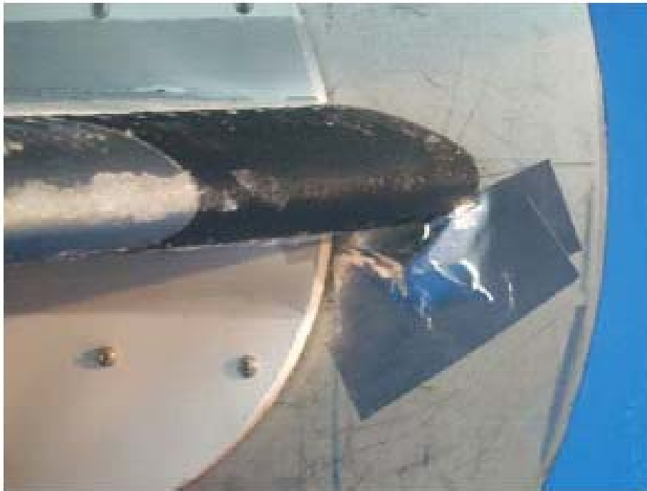
Figure 3-13: Airfoil after being in the icing wind tunnel for approximately 12 minutes at -15^{\circ}\text{C} ; the coated surface (black) exhibited negligible ice build-up relative to the uncoated steel surface.
