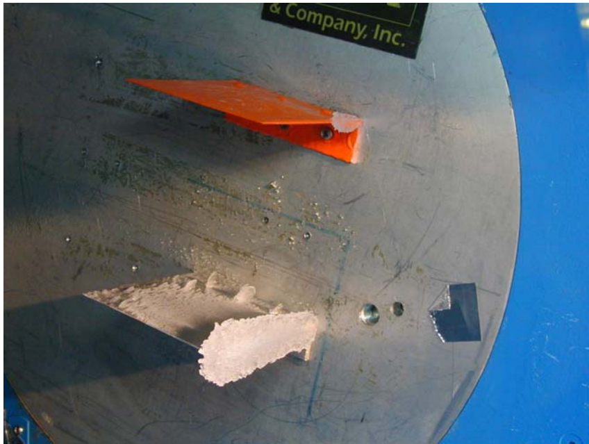
Figure 3-11: Vortex generator after being in the icing wind tunnel for approximately 20 minutes at -2^{\circ}\text{C} ; the coated surface (orange) exhibited negligible ice build-up relative to the uncoated steel surface
