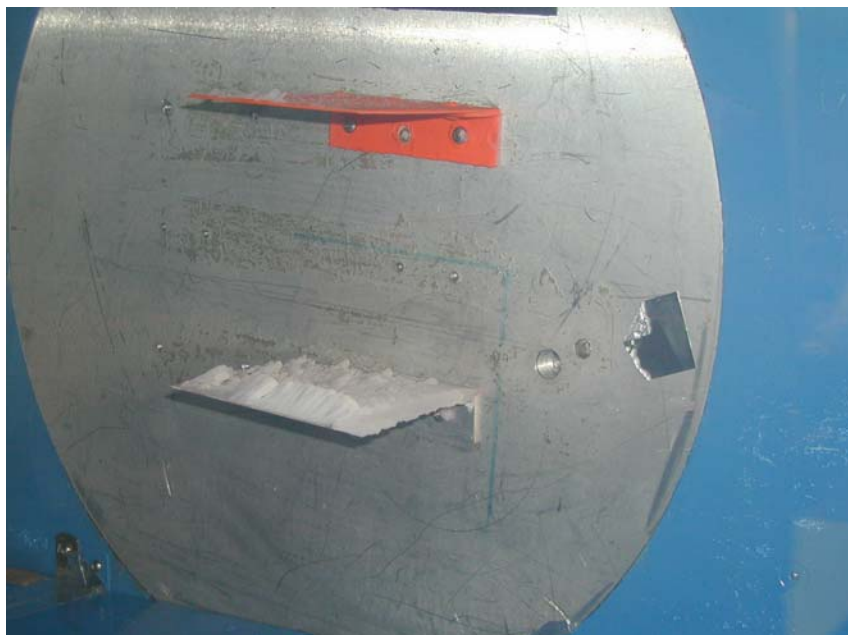
Figure 3-12: Vortex generator after being in the icing wind tunnel for only a few minutes at -9^{\circ}\text{C} ; the coated surface (orange) exhibited negligible ice build-up relative to the uncoated steel surface.
