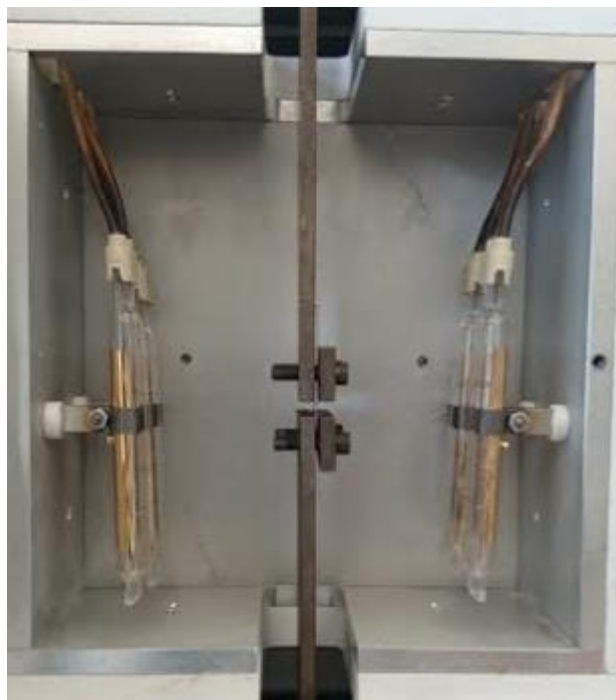
Figure S3.1. Experimental setup for programming strain in polymer sheets in an extensometer. There are two metal grips in the center of the oven that pull the sample vertically while the four infrared lamps control the temperature with an error of \pm 1^\circ\text{C} . The metal grips each have two screws that secure the sample.
