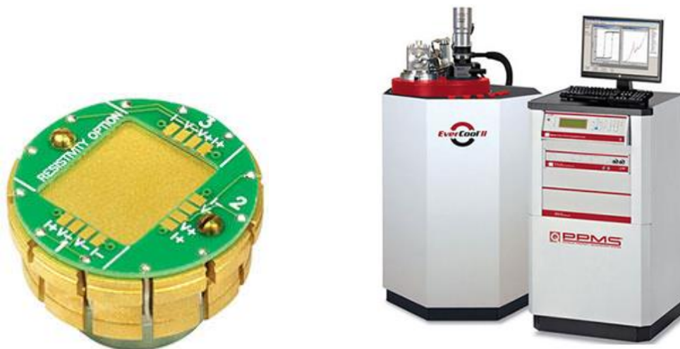
Figure 2.5 (On the left) Picture of a sample puck where our samples are mounted. (On the right) physical property measurement system by quantum design. (Quantum Design Inc) [4]
