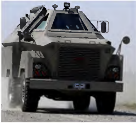
Figure 7. Example of a MRAP vehicle portraying the slant on the front and side of the vehicle.
