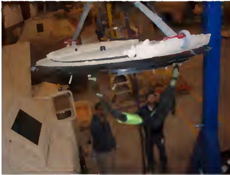
Step 4: Hoist hatch, lower onto geared ring
