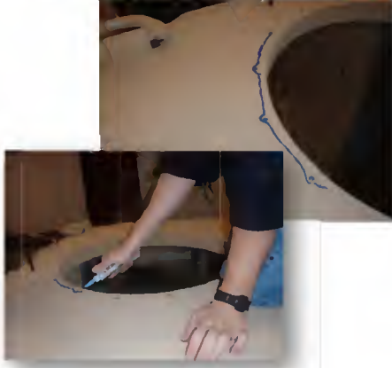
Step 2: Place loctite bead an inch from hatch opening
