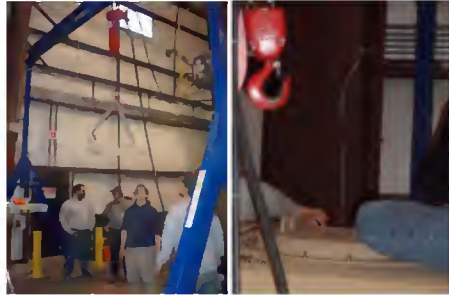
Step 3: Hoist rear turret, line up with holes, secure
