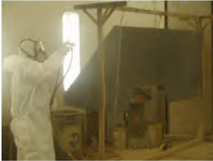
Figure 17. The picture above depicts the painting of a vehicle part.
