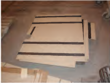
Step 2: Place rear plate, align, secure with bolts
