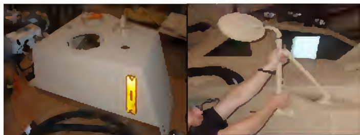
Figure 20. The picture on the left depicts a DOT light box prior to installation. The picture on the right depicts the installation of a mirror onto the vehicle.
