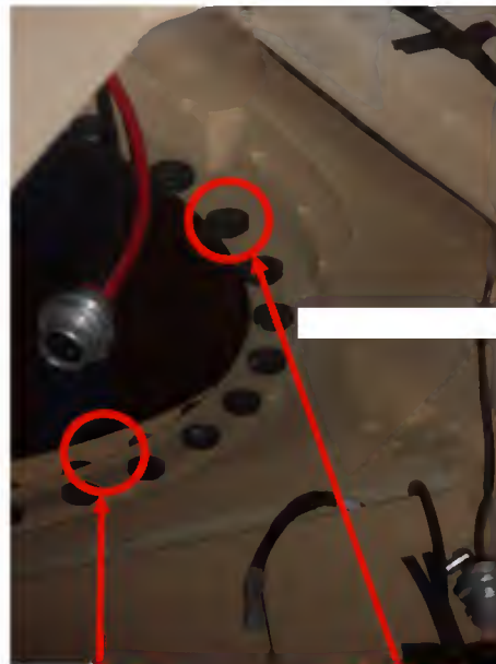
Step 2: Place rubber bushings and sealant foam in holes surrounding the hatch opening
