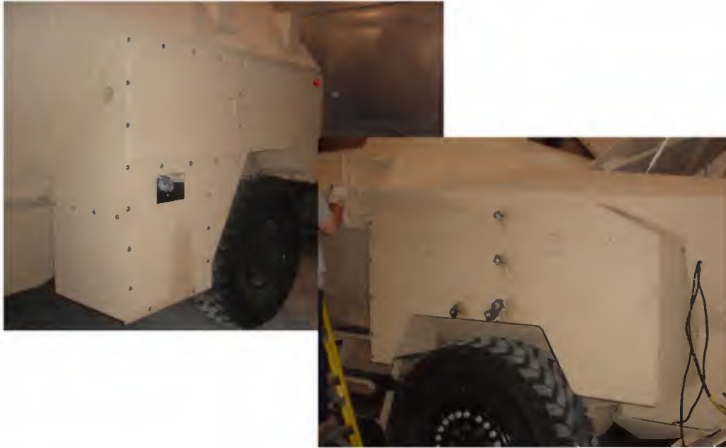
Station 10 Process 1 – Blast Skirts
