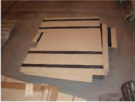
Step 2: Place front floor plate, line up holes, secure with bolts
