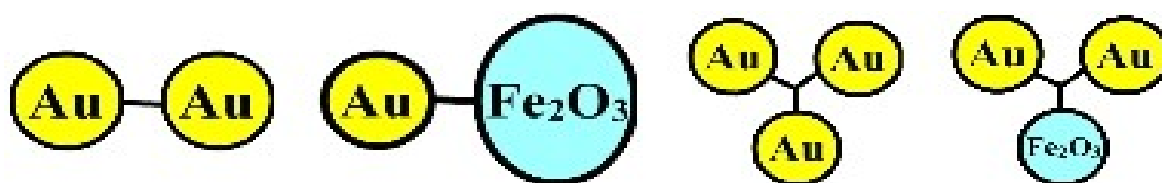
Figure 18. A cartoon of the definition of (from left to right) homo-dimer, hetero-dimer, homo-trimer, and hetero-trimer.
