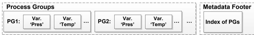
Figure 5.1 The PG data layout in an ADIOS file. Variables are partitioned by PG’s according to which process produced which chunk.
