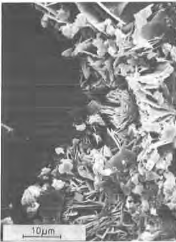
fig. 8: SEM-micrographs of quartz particles in sealed Rhine river gravel concrete after temperature exposure ( T = 180^\circ\text{C} , 40 days).
