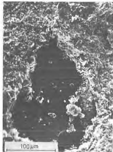
fig. 8: SEM-micrographs of quartz particles in sealed Rhine river gravel concrete after temperature exposure ( T = 180^\circ\text{C} , 40 days).
