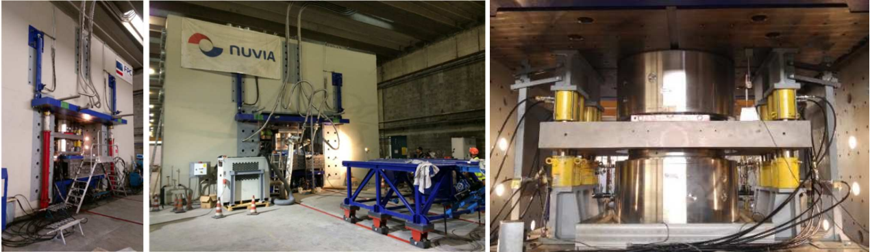
Figure 11. 70MN testing bed for the scale 1 prototype testing
