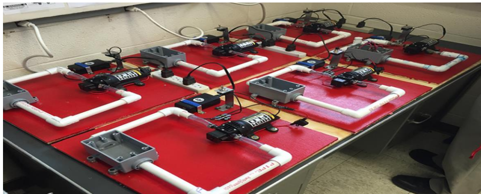
Figure 5. Salt-brine circulator system for corrosion testing.
