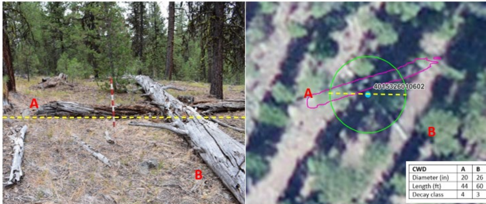
Figure 8. (Left) Photo of field transect looking N with yellow dotted line representing transect. (Right) Aerial imagery of same field transect. Green circle is subplot diameter. Blue dot is transect center. Pink is detected object from DL model. A and B highlight the same two logs visible in each frame with field transect information in bottom right.
