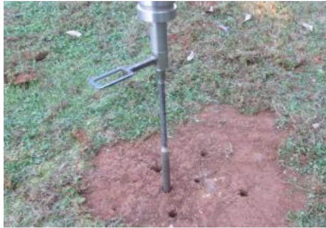
Figure 7.7 MDPT tests at different points (Wake Co. field work).
