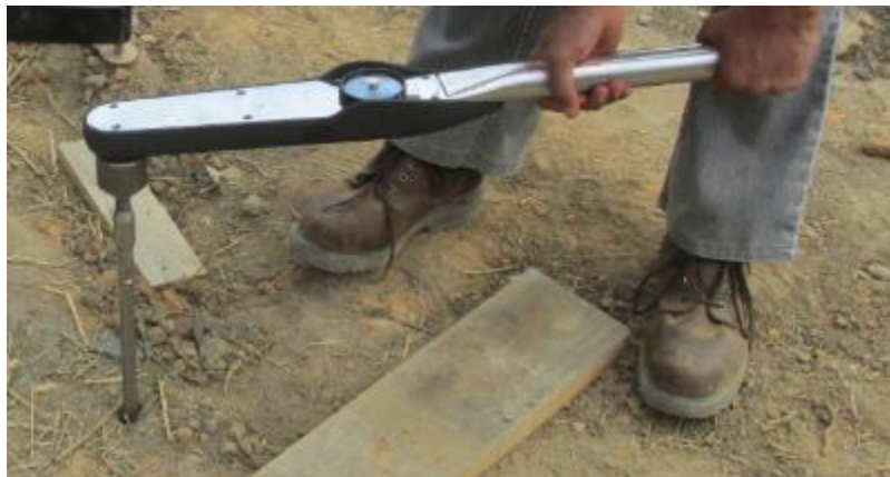
Figure 4.6 Torque wrench to estimate unit skin friction.
