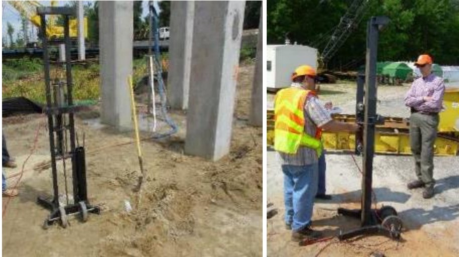
Figure 3.6 Field testing of MDPT in different sites.
