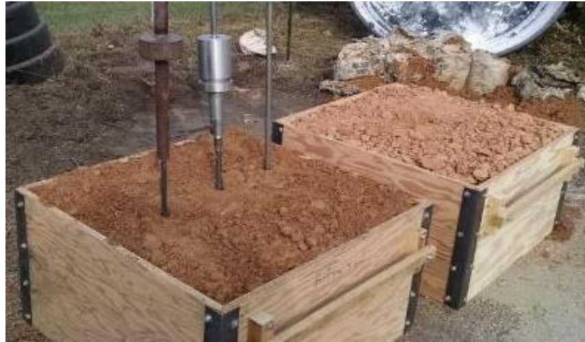
Figure 7.8 Laboratory density tests (MDPT, 0.5 in rod and DCP).
