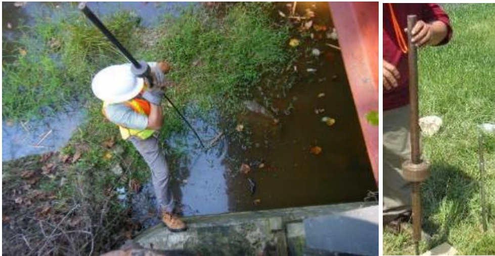
Figure 3.2 In-situ testing using 0.5-in steel rod device to estimate rock elevation.
