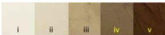
Figure 3.2. Images of composite GO-PAN electrospun fibers with (i) 0 (ii) 1 (iii) 5 (iv) 10 and (v) 20 wt% GO. As GO loading increases, the fiber mats darken.
