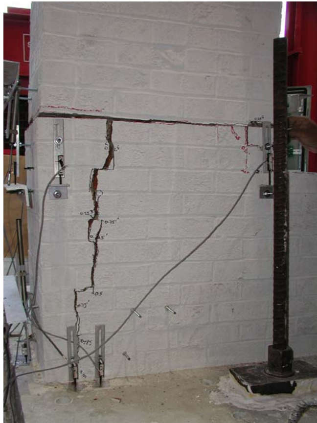
Figure 4: Excessive Crack Width at 1.25 Drift Ratio
