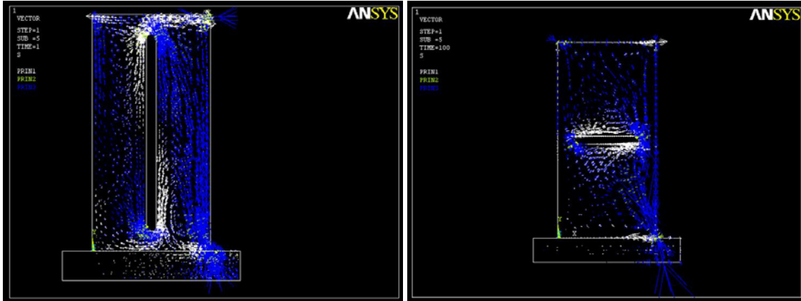
Figure 3: Effect of Openings on Compression Strut
