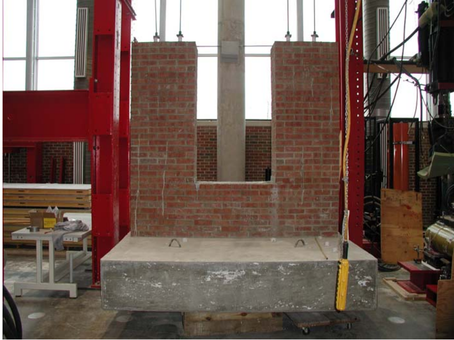
Figure 1: Construction of Masonry Wall with Opening
