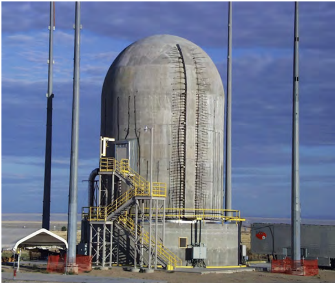
Figure 1. 1:4-Scale Model of a Pre-stressed Concrete Containment Vessel Located at Sandia National Laboratory
