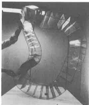
Fig. 7: Master model for one of the nonplanar coils.
