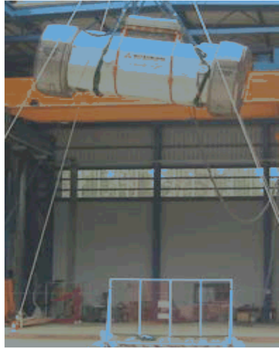
Figure 2. 9-Meter Oblique Drop Cask
