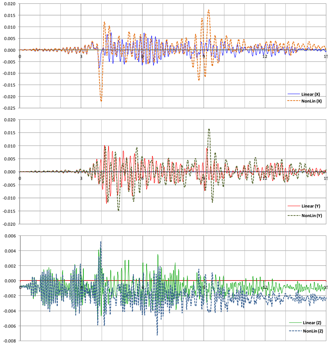
Figure 4: Relative displacements comparison – 0.50g, 4 th floor (Node 647925) [units are sec and m]
