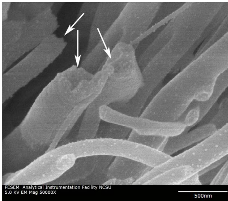
Figure 4.12: SEM image of cross section of electrospun fibers derived from s(8\text{PAA}/\text{DMF})c(5\text{CS}/\text{dHCl})
