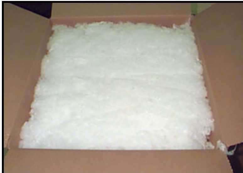
FIGURE 4: Actual Picture of a Feed Matt Sample in a 18x18" Cardboard Box
