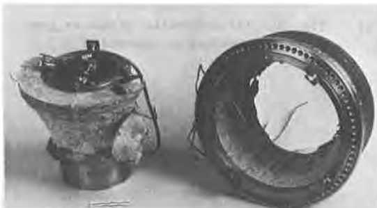
Fig. 5. Posttest view of inner and outer failed sections of the half-thickness model.
