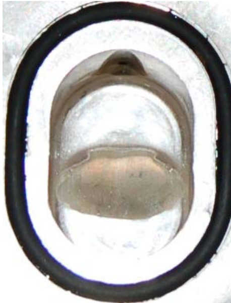
Figure 6-29: TS7 Silver Insert Post-Irradiation
