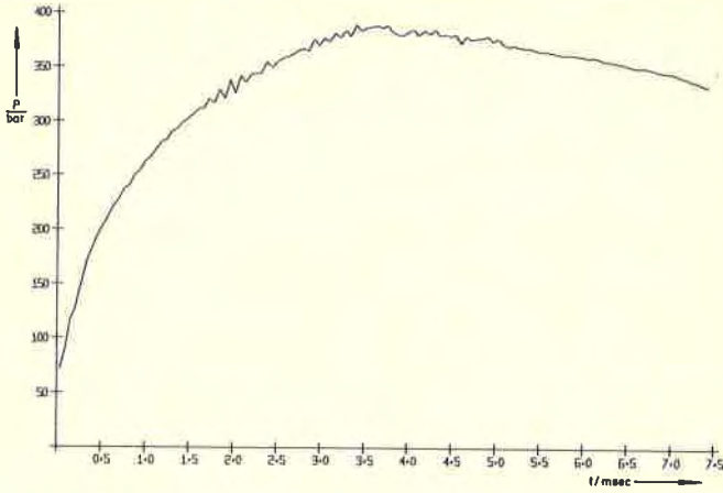
Fig.1: Pressure-time history of FSI; duration of mixing process 4.5 msec
