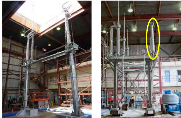
Figure 1. Seismic qualification shaking table tests of 550 kV (left) and 230 kV (right) disconnect switches
