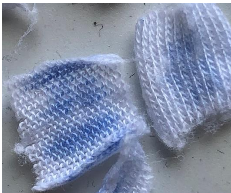
Figure 4.6.1.3 Image of a 50/50 white polyester/blue dyed cotton fabric with partial cotton removal, visually displaying cotton fiber loss from the edges to the middle. Not used for analytical techniques.
