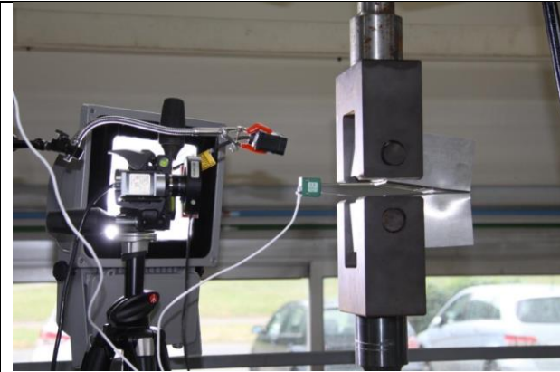
Figure 7: View of the testing equipment for room temperature tests on CT60 specimens
