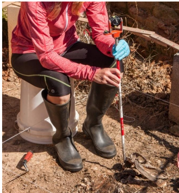
Figure 3.7: The Smaller Prism can be Operated by One Person
