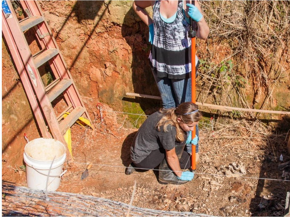
Figure 3.6: The Long Prism must be Operated by Two People
