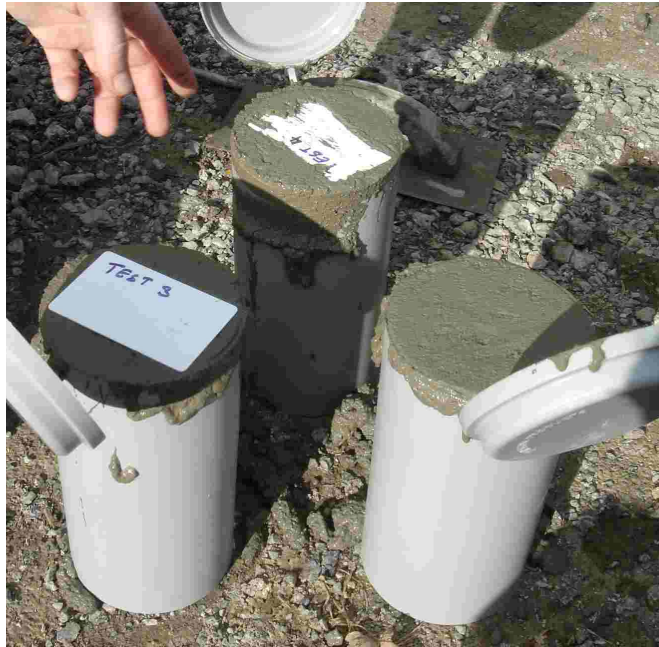
Figure 5.7 Placing plastic RFID tags
