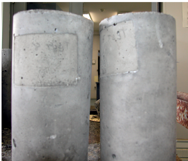
Figure 5.6 Indentation on outer surface of a cylinder due to RFID tags
