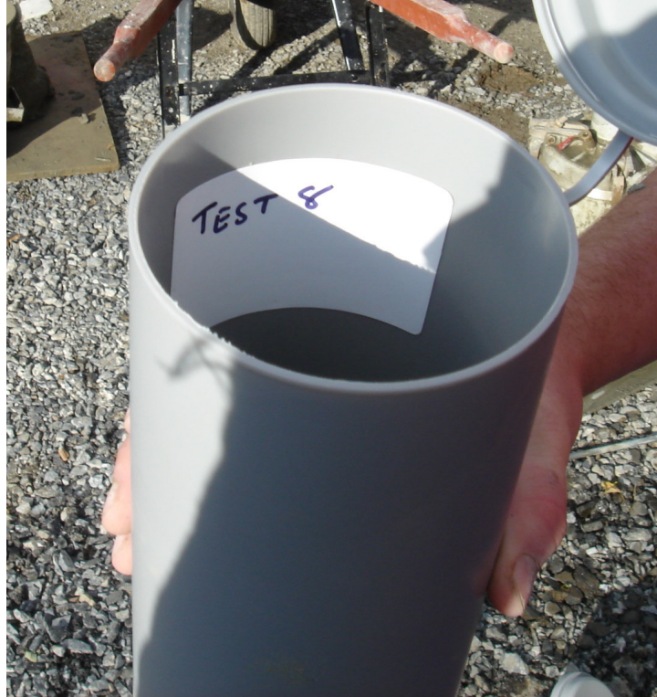
Figure 5.4 RFID tag on inner surface of a cylinder
