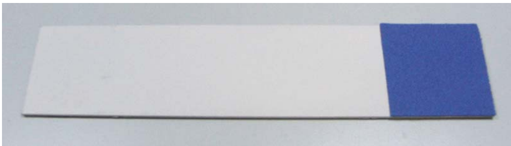
Figure 37. Front side of a sample mount including dyed sample.
