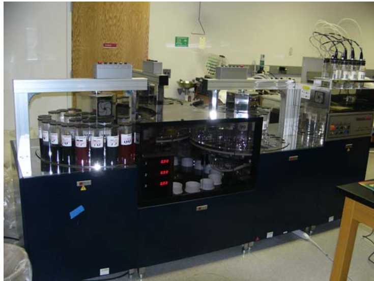
Figure 33. Laboratory Dispenser AutoLab Modulo GT 108/100.
