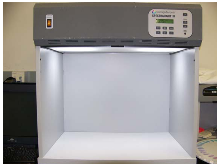
Figure 43. Light booth with D65 illuminant.
