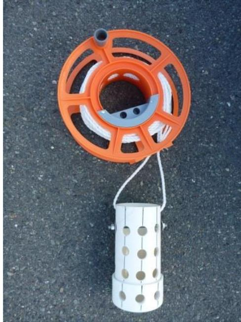
**Figure 3. Bridge sampler for collecting river samples in this study. Glass sample bottles were placed into the perforated pipe and secured with a steel rod.**
