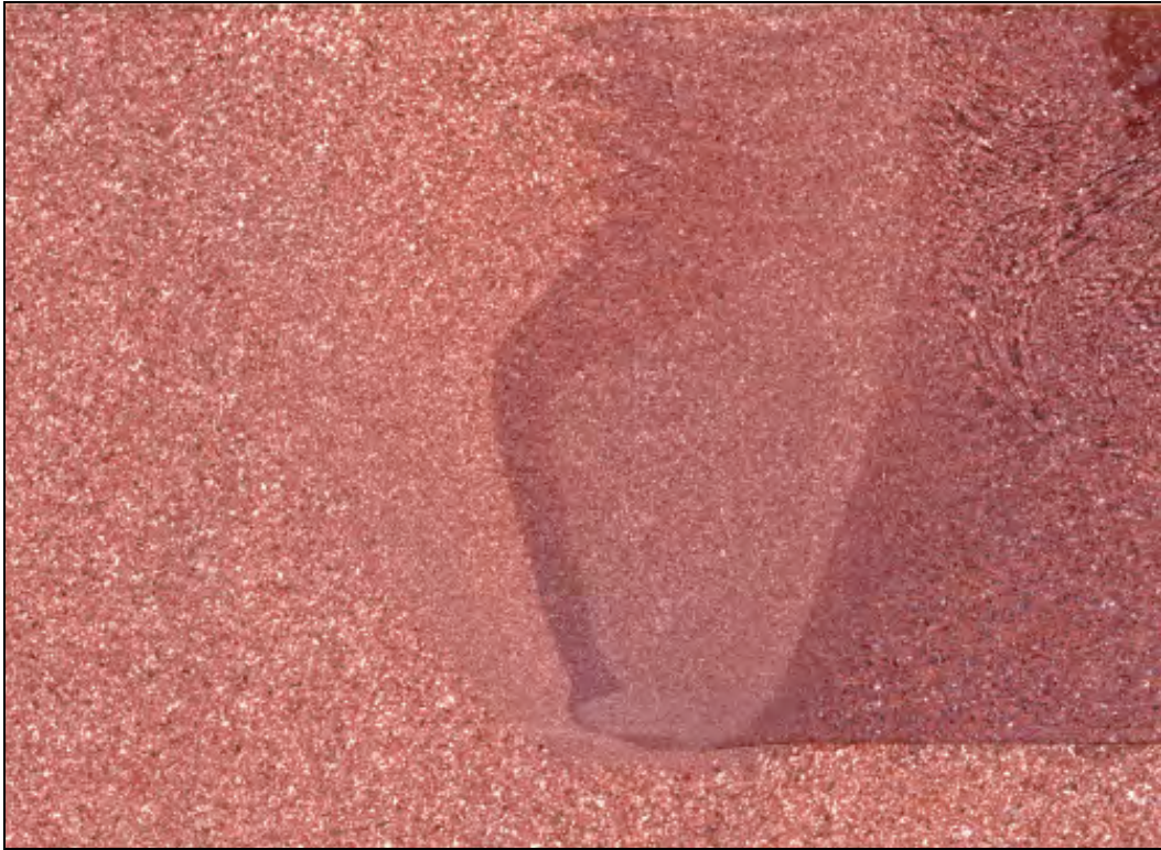
Figure 1. Macrograph of the transverse section of an FS weld. Tube material is on the right side and lid material on the left side. Different zones of the weld can be clearly seen.
