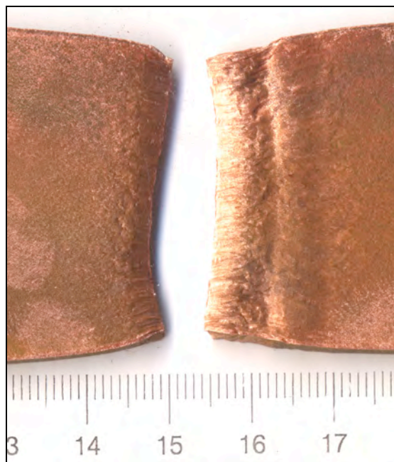
Figure 9. EB weld after tensile testing. The weld has fractured between the weld and the forged lid material due to large grain size gradient. Deformation has also localized at the weld centre with large grains and slightly also between the weld and the extruded tube material where the grain size gradient is less dramatic.
