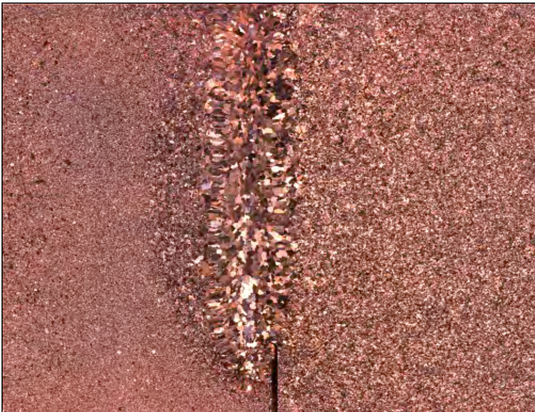
Figure 2. Macrograph of the transverse section of an EB weld. Tube material is on the left side and lid material on the right side. The large grain size of the weld can be clearly seen.
