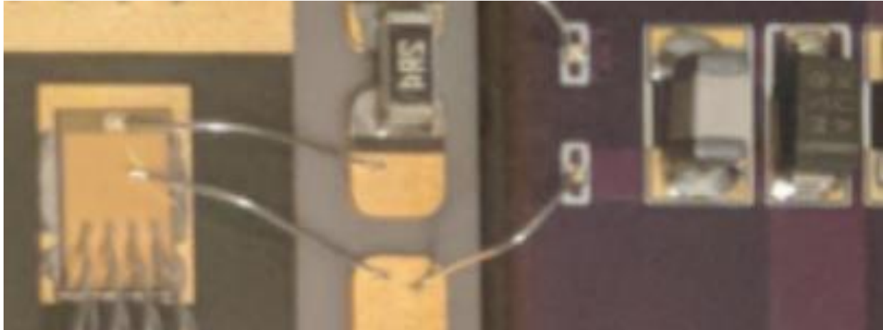
Figure 2.9: Size comparison between a power JFET die (gold on the left) and a packaged avalanche diode (black on the right), estimated die size of the avalanche diode is 1/6 of its package size
