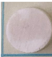
Figure 6.14 Coloration in 1 kHz flash sintered YSZ.
