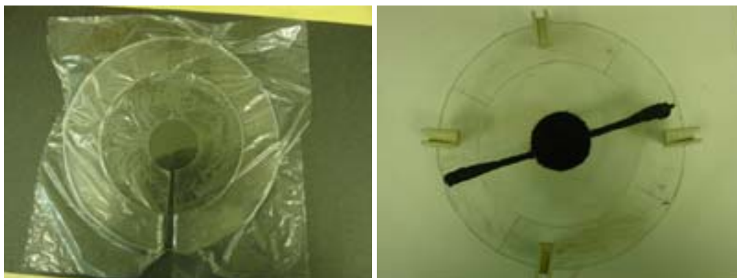
Figure 31: a) Film with mask b) Final actuator
