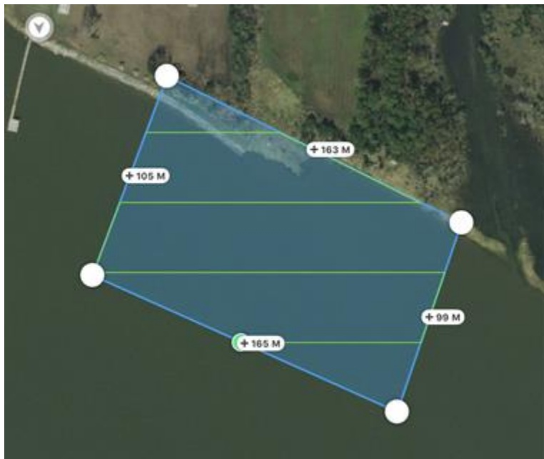
Figure 9: Flight plan over the study site generated in the DJI GS Pro (2.0.15) app
