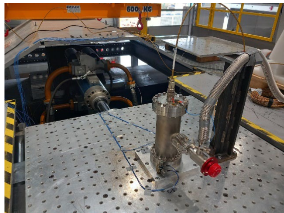
b- View of a specimen seismically qualified
