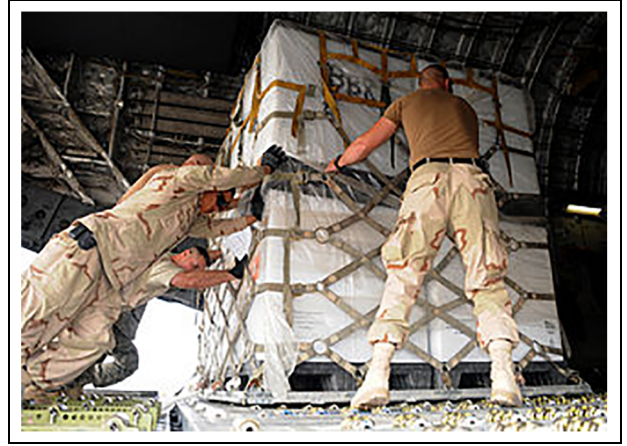
Figure 7. Depiction of a 463L pallet with multipack containers in Al Taqqadum, Iraq (9 January 2009). Seabees assigned to Naval Mobile Construction Battalion 7 and airmen of the Air Force Expeditionary Logistics Readiness Squadron Detachment 4 maneuver 463L pallets into an Air Force C-17 for transportation. 59
