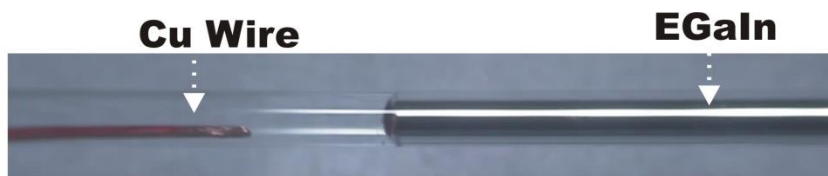
Figure S4. Effect of electrical length on withdrawal velocity. A copper wire (anode) was inserted into the capillary to shorten the electrical distance between the anode and the metal interface. Shortening the distance increases the velocity for a given voltage.
