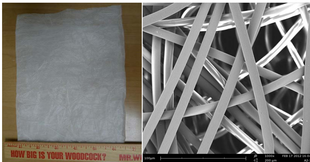
Figure 3.2. (a) Optical image of scoured nonwoven PLA fabric; (b) SEM image of scoured nonwoven PLA fabric
