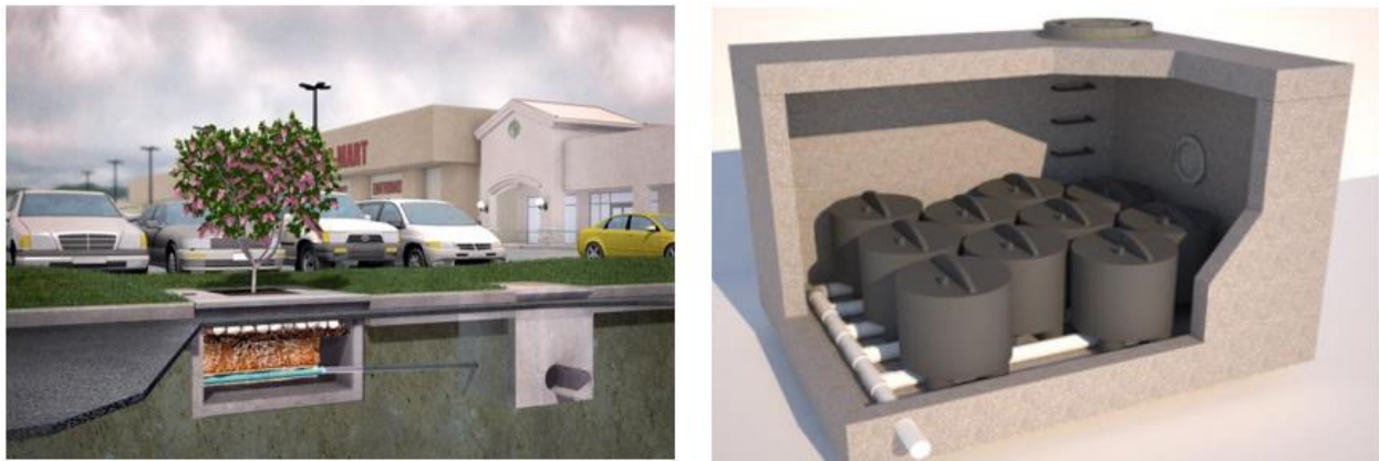
Figure 1-3. Schematic of two vaulted MTDs: Contech’s Filtterra ® (left) is a vaulted biofiltration system and Advanced Drainage System’s (ADS) BayFilter ® (right) is a vault cartridge filtration system. Source: NCDEQ, (2017).
