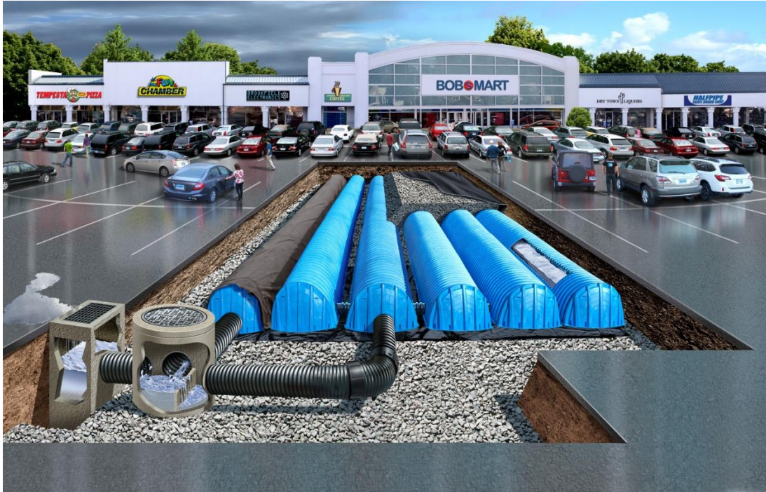
Figure 1-4. Schematic of a subsurface detention MTD: Cultec’s Contactor® and Recharger®. (Image courtesy Cultec).
