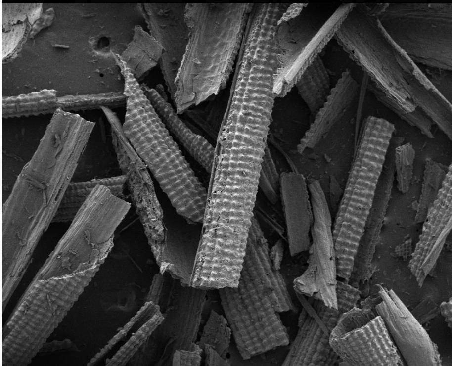
Figure 4. Surface view of (A) rice hulls (RH) and (B) rice hull biochar (RBC) at 30x magnification.
