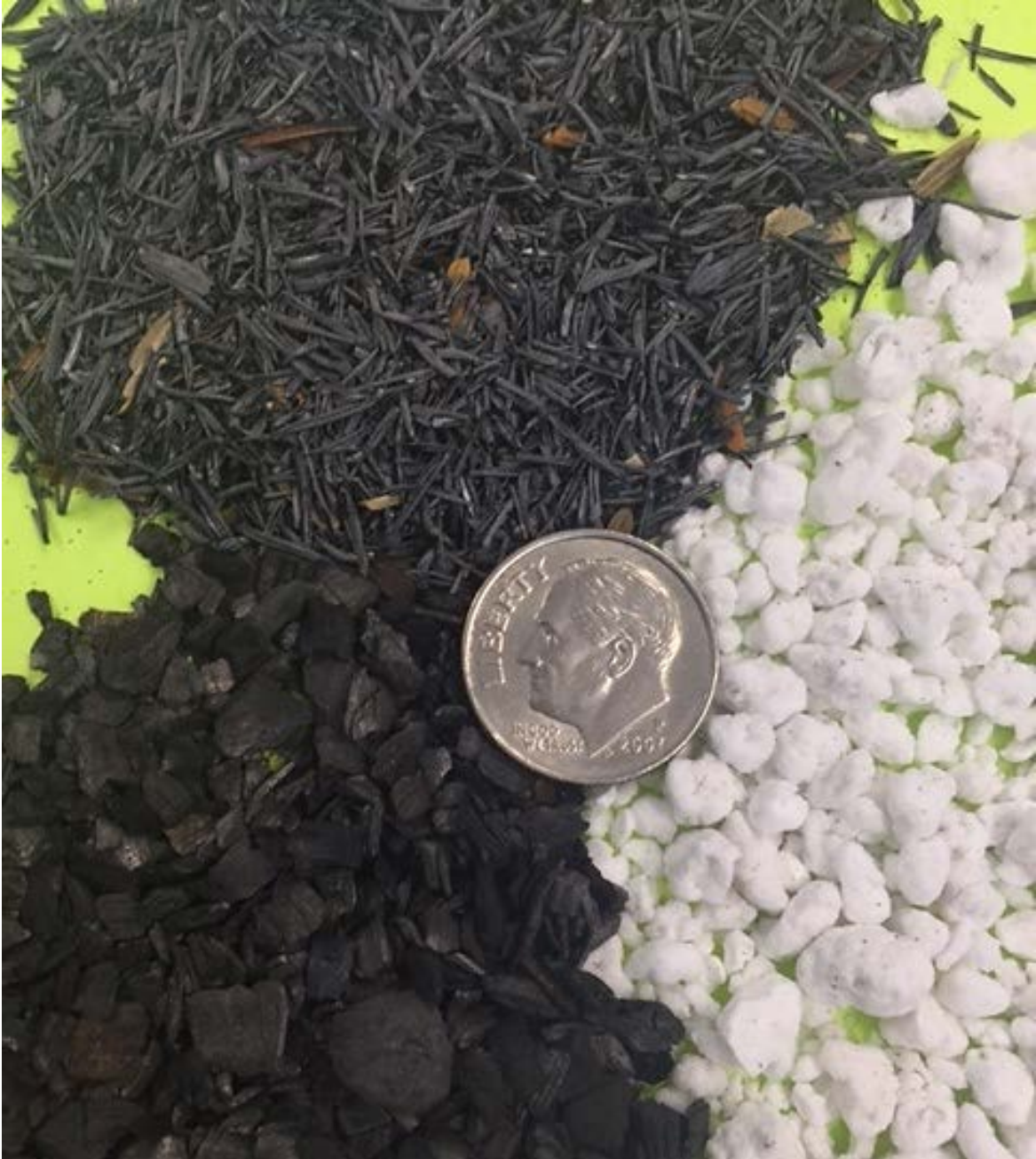
Figure 4. Comparison of particle size and shape of rice hull biochar (RBC), perlite (PL) and pine wood biochar (PBC).
