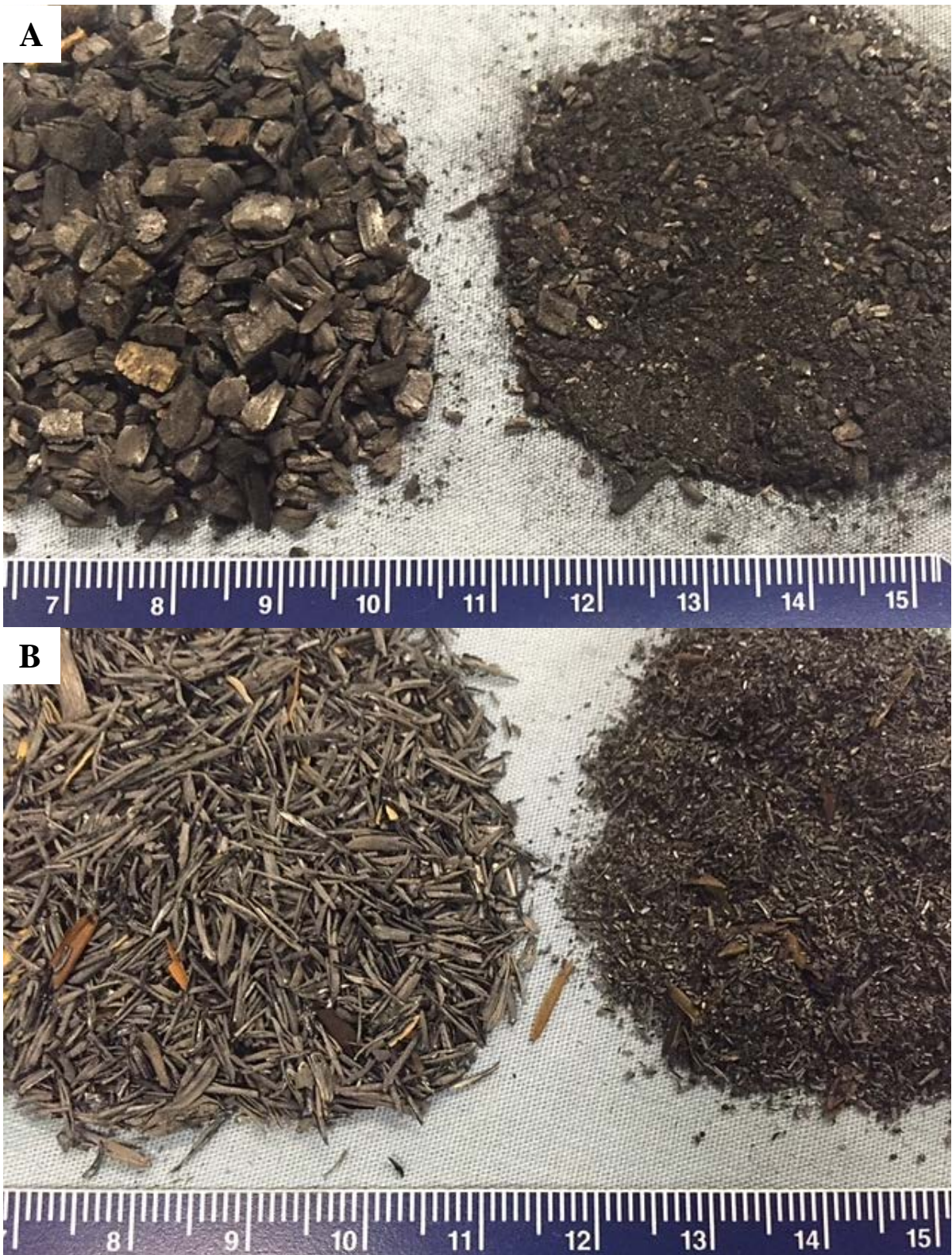
Figure 2. (A) On the left, biochar produced from pine wood (loblolly; Pinus taeda ), that was then ground to <2-mm size (right; PBC p ). (B) On the left, biochar produced from rice hulls, that was then ground to <2-mm size (right; RBC p ).
