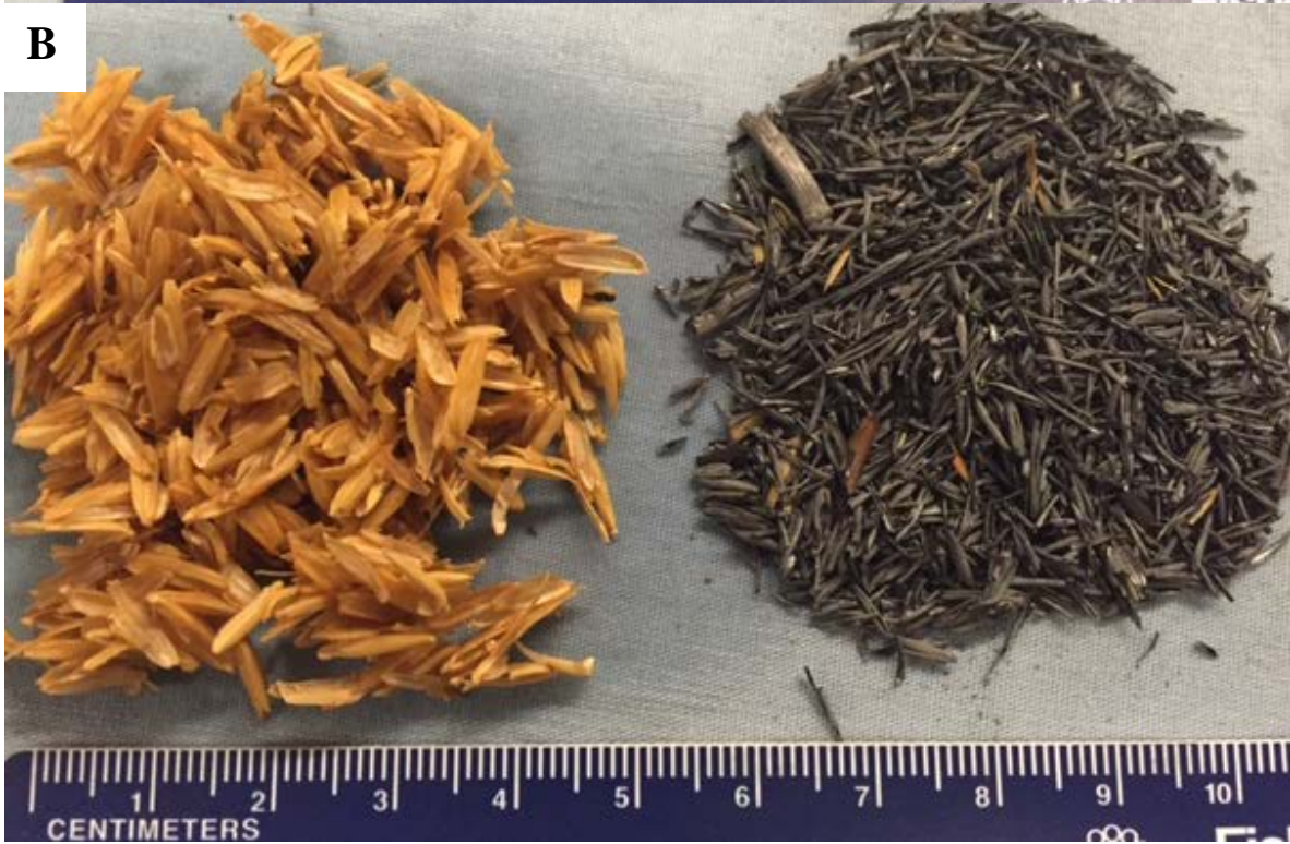
Figure 2. (A) On the left, pine wood chips feedstock (loblolly pine; Pinus taeda ) and final pine wood biochar product (right) made using the top-lit updraft (TLUD) gasifier. (B) On the left, rice hull feedstock and final rice hull biochar product (right).
