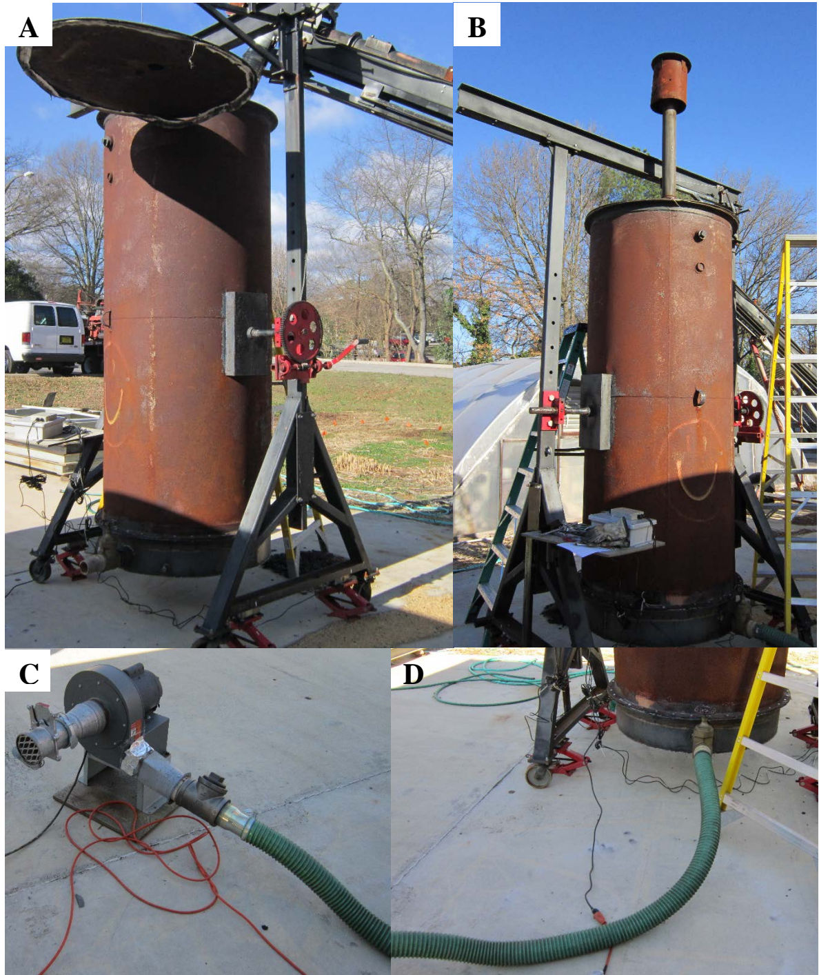
Figure 1. (A) Top-lit updraft (TLUD) gasifier used to produce pine wood chip and rice hull biochars. (B) Gasifier with lid and gas stock attached to show entire system. (C) The air fan used to blow 12\text{-m}^3\cdot\text{min}^{-1} and (D) the connecting tube connected to the bottom of the gasifier to force air up.
