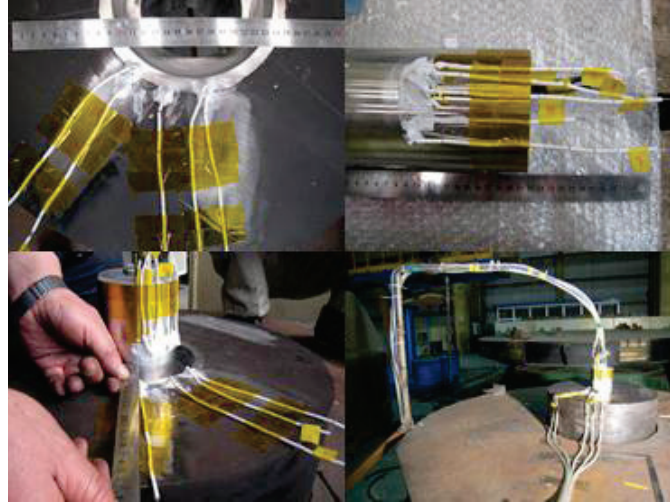
Figure 4. Sensors installation and wire layout
