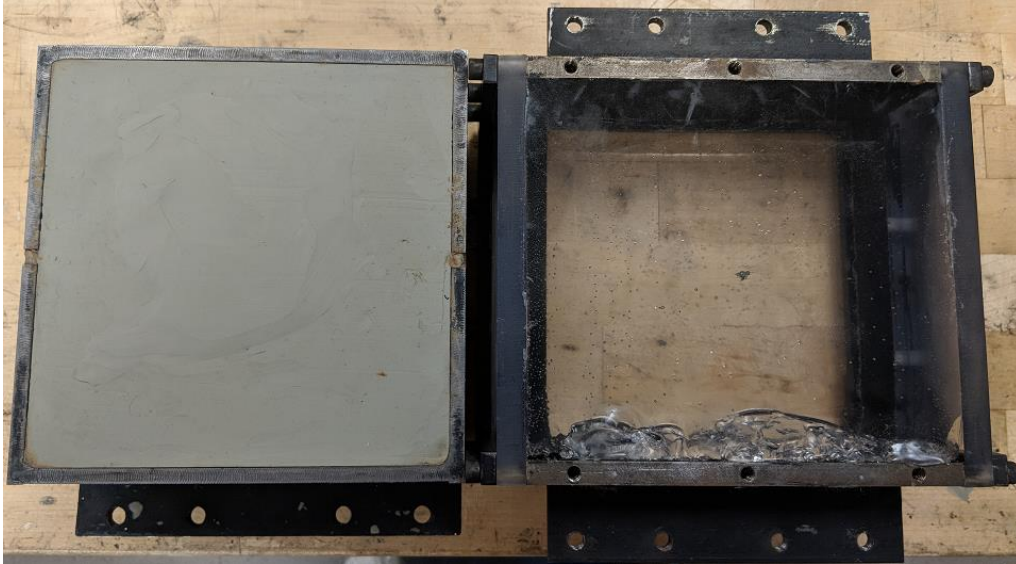
Figure 10: (Left) Roma Plastilina #1 Modeling Clay and (Right) 20% Ballistics Gelatin.
