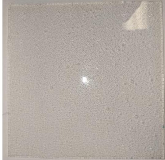
Figure 31: Sorta-Clear Sample With Large Amount of Trapped Air.
