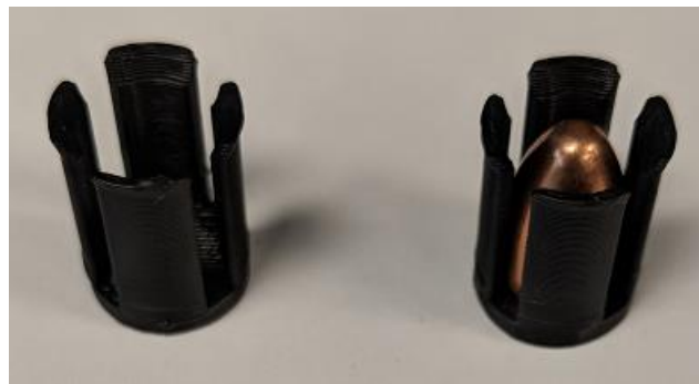
Figure 6: (Left) 9mm Sabot and (Right) Sabot with Mounted 9mm Projectile.
