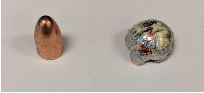
Figure 4: (Left) Undeformed Projectile and (Right) Projectile After Impact.
