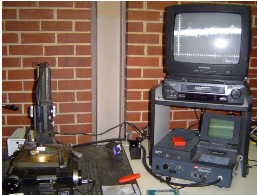
Fig. 3.6. Apparatus for measuring the cutting edge sharpness.
